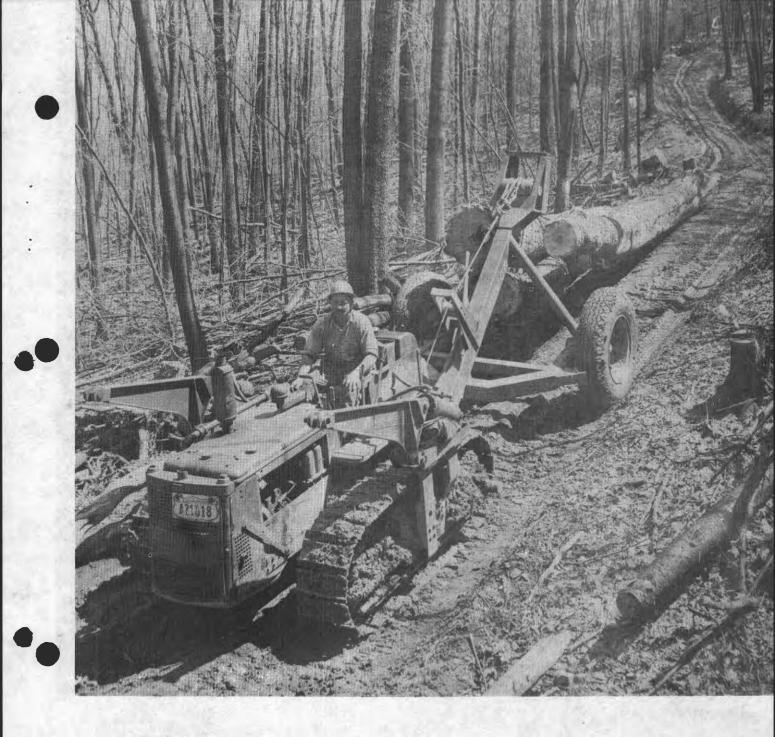
With well-planned skid roads, modern equipment like the tractor-winch-arch combination can be used efficiently for mountain logging.
