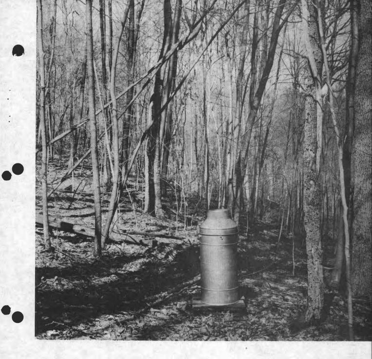
How does forest vegetation affect watershed management? In one study, rain gages like this are used to determine how the tree canopy reduces the force of rain striking the forest floor.
